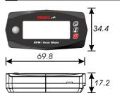
●Digital Tachometer Display range: 0~15,000 RPM
