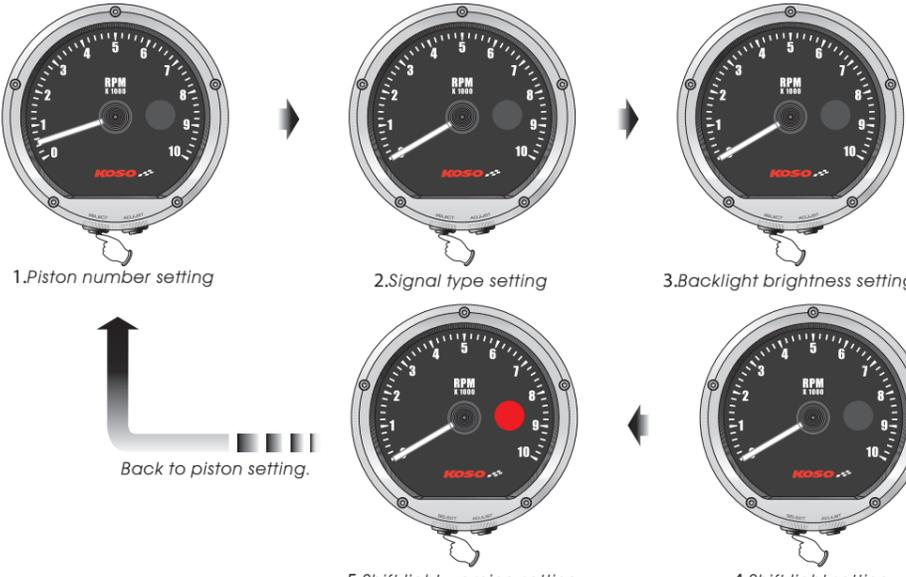
1. Piston number setting      2. Signal type setting      3. Backlight brightness setting
