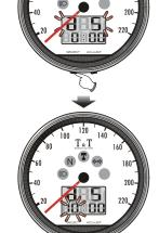
●EX. To change the setting to 10:00. ●Press the Adjust button to choose the setting
