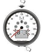
Press the Adjust button once to go back to the tire circumference and sensor point setting screen.
