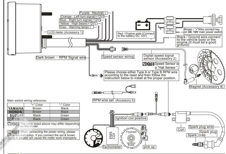
When connecting the power wiring, please follow the instruction. If you connect the red & brown wiring in parallel will cause the meter work improperly.
