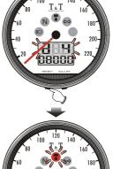
●EX: You want the shift light to light on at 8000 RPM Please change the shift light setting value to 8500 directly.
