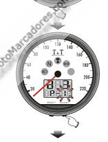
●Enter the number of ignition signals per crankshaft revolution ("P" value). This may vary according to the vehicle manufacturer/model and type of engine:
