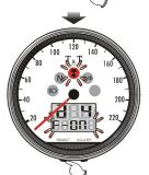
Press the Select button once to go back to the RPM input signal and shiftlight setting
